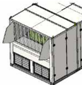
Step 2: Position side flange with corner on the outside
