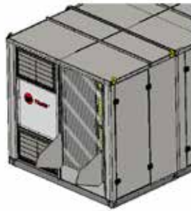
Step 2: Position side flange with corner on the outside
