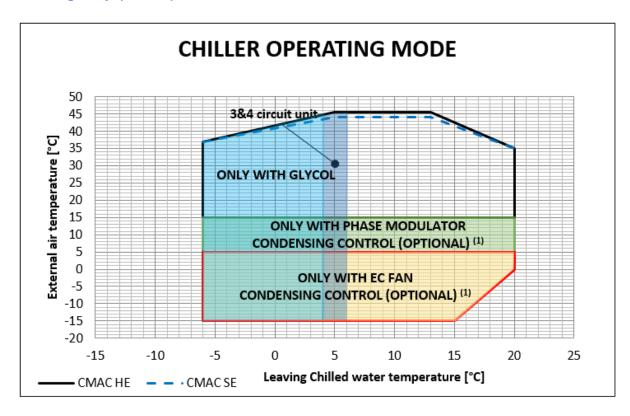
(1) In this area the fans modulate in order to control the condensing/evaporating temperature. The performances may be different from the declared ones.
