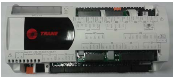
Figure 2 – Trane CH536 controller
