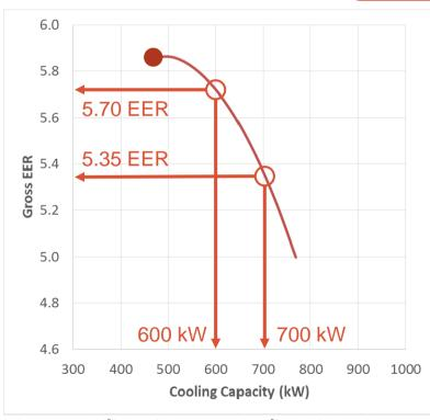
Performance curve at 7/12°C entering /leaving evaporator and 30/35°C entering /leaving condenser
