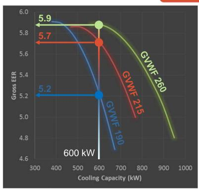
Performance curve at 7/12°C entering /leaving evaporator and 30/35°C entering /leaving condenser
