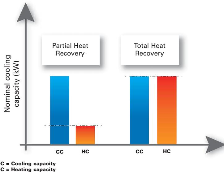
**Partial Heat Recovery:** specifically designed for applications where a limited amount of heat needs to be recovered and actually used in the building. This is, for example, the case of an office or commercial building where heat recovered from the HVAC installation can be used to heat or preheat the sanitary hot water.
