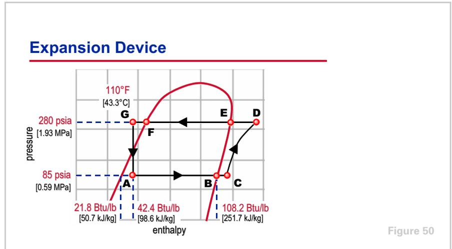
The temperature of the refrigerant entering the expansion device (**G**) is 110°F [43.3°C] and its pressure is 280 psia [1.93 MPa]. (The refrigerant condensed at 121.5°F [49.7°C] and was subcooled to 110°F [43.3°C].) The enthalpy of the refrigerant at this condition is 42.4 Btu/lb [98.6 kJ/kg]. As mentioned previously, there is no change in enthalpy during the expansion process—it is the same at both **G** and **A**.
