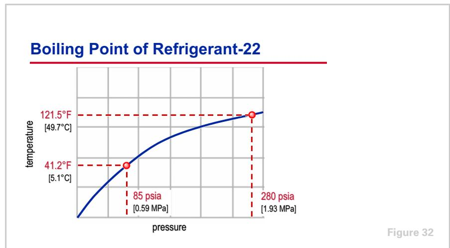
This curve illustrates the pressures and corresponding temperatures at which R-22 boils and condenses. At a pressure of 85 psia [0.59 MPa], the liquid R-22 will boil at 41.2°F [5.1°C]. As an example, assume that a compressor is used to
