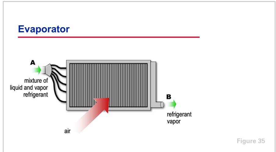
At the inlet to the **evaporator**, the refrigerant exists as a cool, low-pressure mixture of liquid and vapor. In this example, the evaporator is a finned-tube coil used to cool air. Other types of evaporators are used to cool water.
