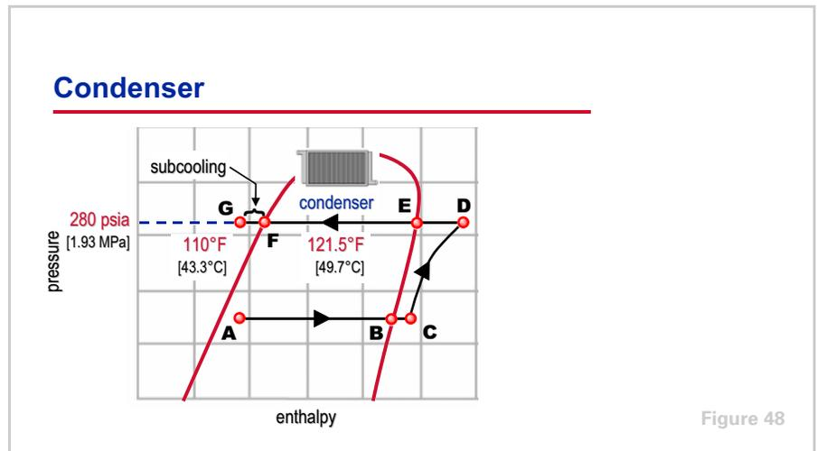
Inside of the condenser, heat is transferred from the hot, high-pressure refrigerant vapor (**D**) to relatively cool ambient air. This reduction in the enthalpy of the refrigerant vapor causes it to desuperheat. It becomes saturated vapor, condenses into saturated liquid, and further subcools before leaving the condenser (**G**) to go to the expansion device.
