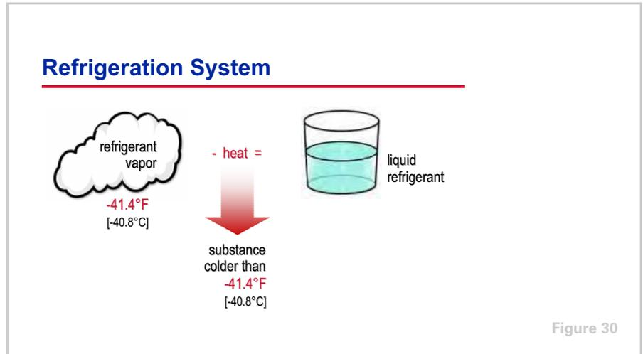
The liquid refrigerant absorbed heat from the air while it was inside the evaporator, and was transformed into a vapor in the process of doing useful cooling. Earlier in this clinic, we demonstrated that if the heat is then removed from this vapor, it will transform (condense) back to its original liquid phase.
