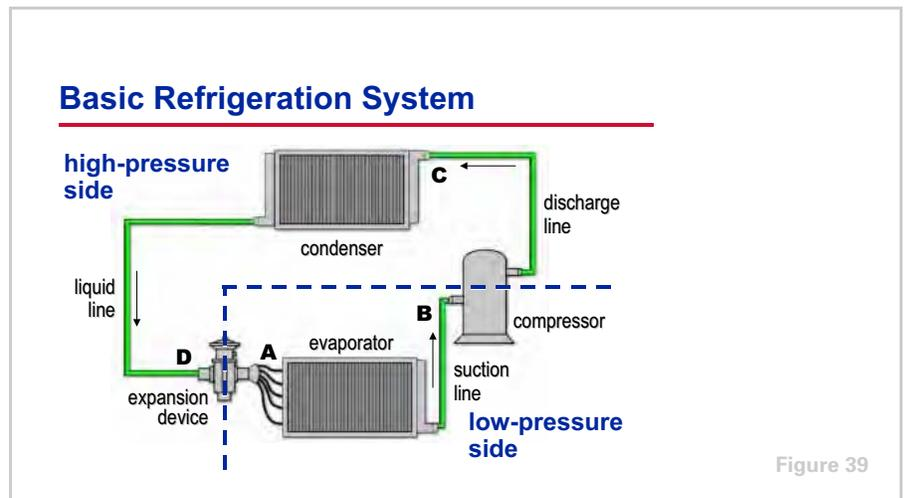
Placing each component in its proper sequence within the system, the compressor and expansion device maintain a pressure difference between the high-pressure side of the system (condenser) and the low-pressure side of the system (evaporator).
