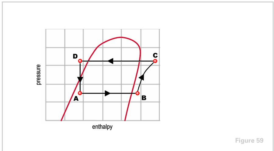
**13** Using the pressure–enthalpy chart in Figure 59, identify the components of the vapor-compression refrigeration cycle:
