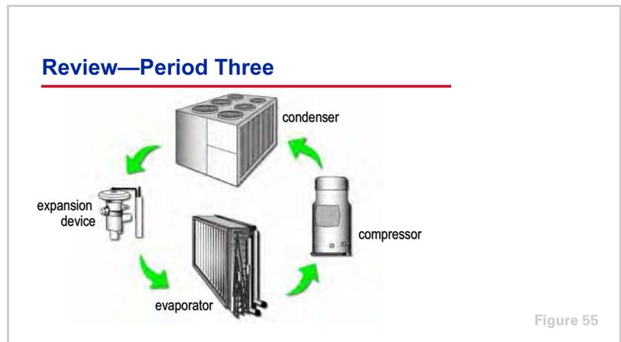
Period Three presented the basic vapor-compression refrigeration cycle, and specifically the use of a compressor, condenser, and expansion device to “recover” the evaporated refrigerant and complete the cycle. The primary components of the vapor-compression refrigeration cycle include the evaporator, compressor, condenser, and expansion device.
