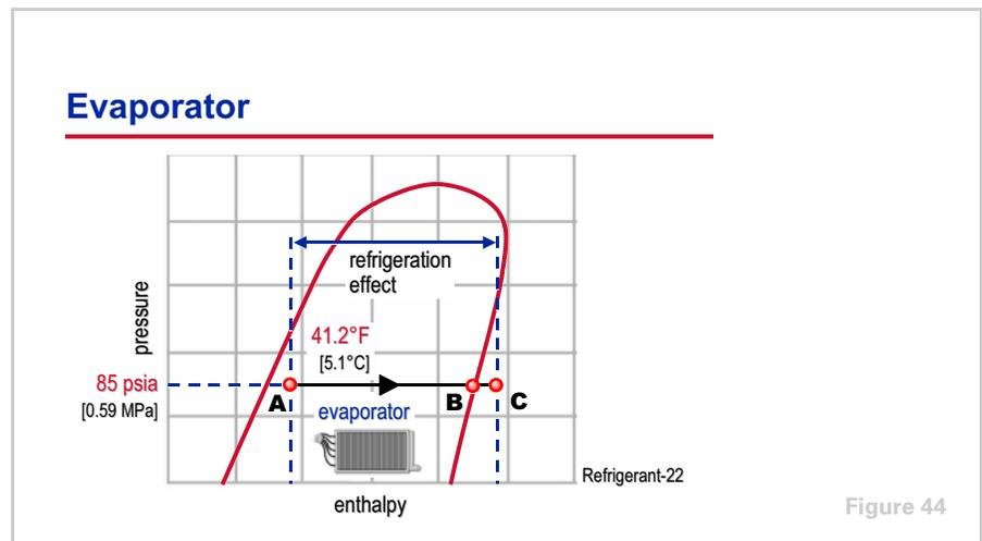
The *P-h* chart can be used to analyze the vapor-compression refrigeration cycle and determine the conditions of the refrigerant at any point in the cycle. The chart in this example is for R-22.
