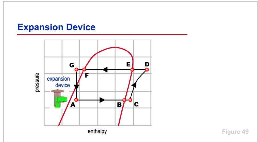
The primary purpose of the expansion device is to drop the pressure of the liquid refrigerant to equal the evaporator pressure. At this lower pressure, the refrigerant is now inside the saturation envelope where it exists as a mixture of liquid and vapor.
