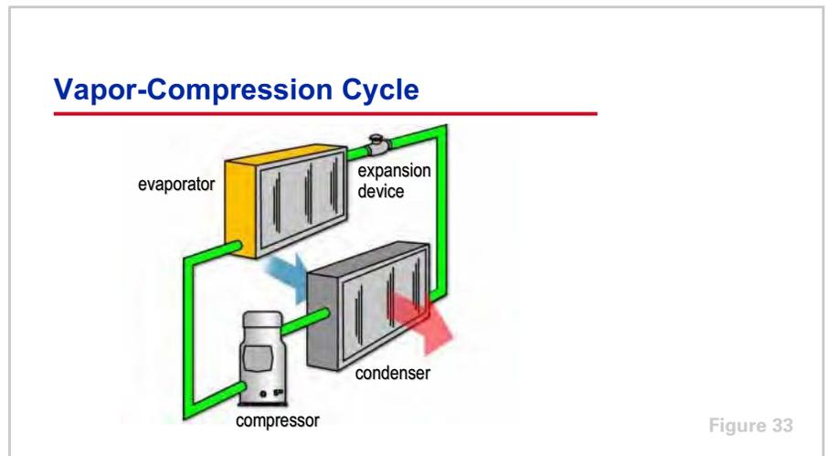
A compressor, condenser, and expansion device form the rest of the system that returns the refrigerant vapor to a low-temperature liquid, which can again be used to produce useful cooling. This cycle is called the **vapor-compression refrigeration cycle**.
