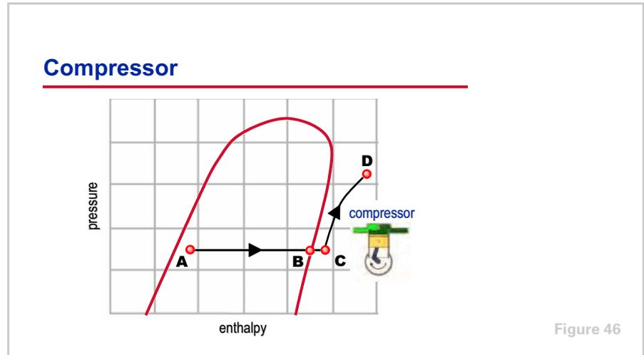
The compressor draws in the superheated refrigerant vapor (**C**) and compresses it to a pressure and temperature (**D**) high enough that it can reject heat to another fluid. As the volume of the refrigerant is reduced by the compressor, its pressure is increased. Additionally, the mechanical energy used by the compressor to accomplish this task is converted to heat energy. This causes the temperature of the refrigerant to also rise as its pressure is increased.
