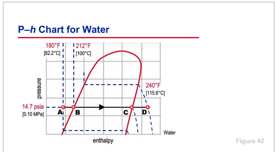
To further demonstrate the use of the P–h chart, let us look at the process of heating and boiling water, at a constant pressure, on a P–h chart for water.
