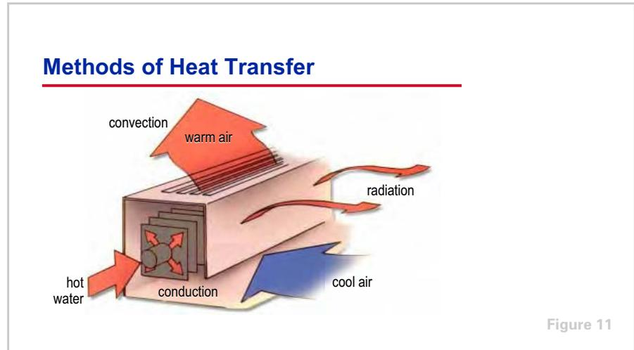
The third principle is that heat is transferred from one substance to another by one of three basic processes: conduction, convection, and radiation. The device shown is a baseboard convector that is commonly used for heating a space. It can be used to demonstrate all three processes of transferring heat.
