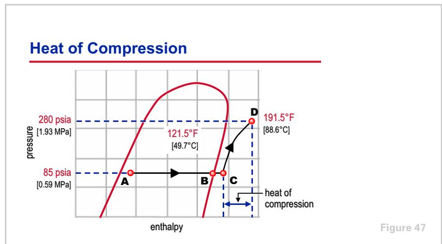
When the refrigerant vapor is discharged from the compressor, its temperature is substantially higher than its saturation temperature (the temperature at which the refrigerant would condense). The increase in enthalpy from **C** to **D** is due to heat added by the compressor, or the **heat of compression**.
