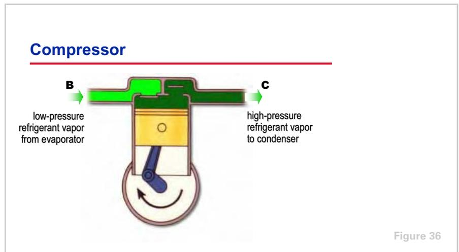
The **compressor** raises the pressure of the refrigerant vapor (**B**) to a pressure and temperature high enough (**C**) so that it can reject heat to another fluid, such as ambient air or water. There are several types of compressors. The type shown in this figure is a reciprocating compressor.
