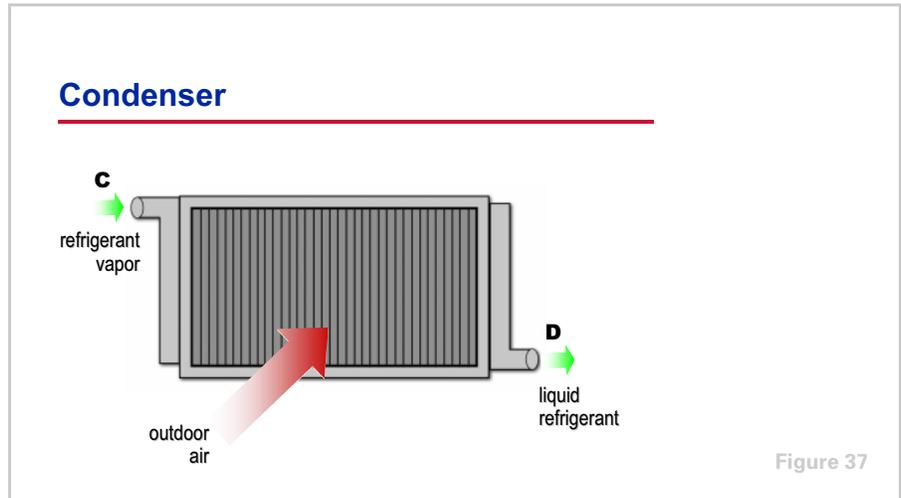
The **condenser** is a heat exchanger used to reject the heat of the refrigerant to another medium. The example shown is an air-cooled condenser that rejects heat to the ambient air. Other types of condensers are used to reject heat to water.
