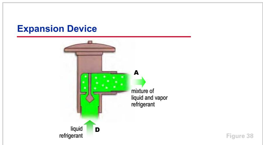
The primary purpose of the **expansion device** is to drop the pressure of the liquid refrigerant to equal the pressure in the evaporator. Several types of expansion devices can be used. The device shown is an expansion valve.
