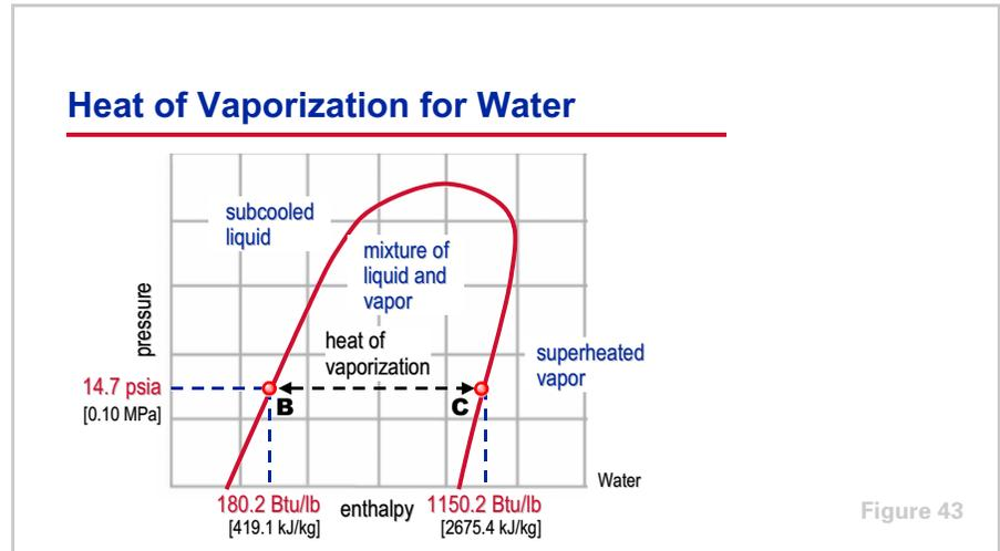
The distance between the edges of the envelope indicates the quantity of heat required to transform saturated liquid into saturated vapor at a given pressure. This is called the **heat of vaporization**.
