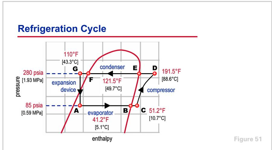
This cool mixture of liquid and vapor refrigerant leaving the expansion device then enters the evaporator (**A**) to repeat the cycle.
