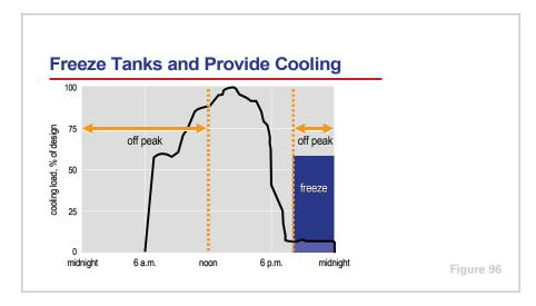
Sometimes, it may be necessary to freeze the water inside the ice storage tanks while simultaneously satisfying a building cooling load. In this example, the time required to freeze all the water inside the tanks is longer than the six-hour period from midnight to 6 a.m. Therefore, the chiller also needs to operate in ice-making mode between 8 p.m. and midnight. During this time, a building cooling load also exists.
