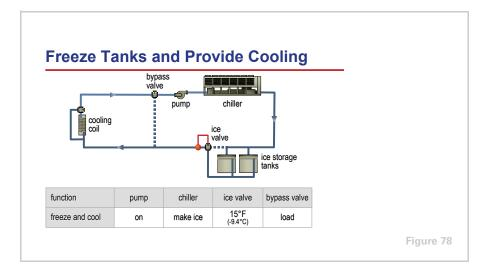
The fifth operating mode is to freeze the water inside the storage tanks and satisfy a simultaneous building cooling load.
