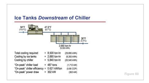
First, consider if the ice storage tanks are located *downstream* of the chiller. This configuration allows the chiller to receive the warmest, entering-fluid temperature, and to produce a higher leaving-fluid temperature. This results in increased chiller capacity and improved efficiency. In this example, the chiller cools the fluid from 58°F (14.4°C) to 47.6°F (8.7°C), at an efficiency of 0.621 kW/ton (5.66 COP).
