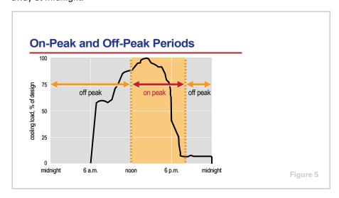
Most electric utility companies experience the greatest demand for electricity during the daytime hours, with some even facing capacity shortages. To encourage the reduction of electricity use during these times, many electric
