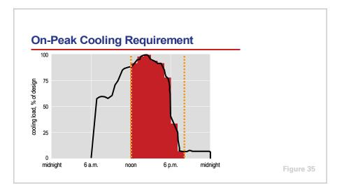
Two different cooling-load profiles are helpful when determining the ice storage capacity of the system. The first is the 24-hour cooling-load profile for the design day. This is useful for balancing chiller capacity, tank freeze rate, and tank melt rate to ensure that the cooling loads can be satisfied for each hour of the design (or worst-case) day.
