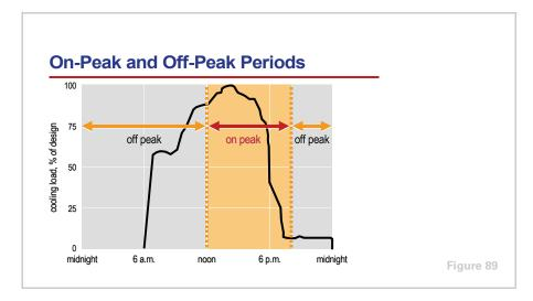
In many buildings, the thermal load is the result of building occupancy and function. Therefore, the times and days at which these loads occur are typically repetitive. Figure 89 shows the example design-day cooling-load profile introduced in Period One. The peak cooling loads for this example building occur between 11 a.m. and 4 p.m.
