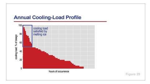
The second cooling-load profile that is helpful for determining ice storage capacity is the annual cooling-load profile. This chart displays how the building cooling load (on the Y axis) varies throughout the year, and the total number of hours (on the X axis) each load occurs. This profile can be useful to balance the installed cost of the storage tanks with the utility-cost savings.
