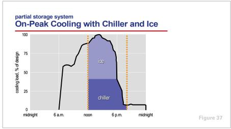
On the design day, a partial-storage system uses both the chiller and the ice storage tanks to satisfy the on-peak cooling requirement. The chiller operates at a reduced capacity, and the cooling loads above this capacity are satisfied by melting ice. On less-severe (or part load) days, however, the system may have sufficient storage capacity to satisfy the entire on-peak cooling requirement by melting the ice only.
