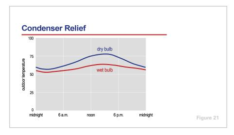
Fortunately, however, the capacity and efficiency loss is generally less severe because the temperature (and, therefore, the pressure) of the refrigerant inside the chiller condenser is typically lower when the chiller is operating in icemaking mode.
