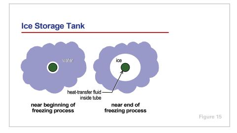
The effectiveness of heat transfer inside a static ice storage tank varies throughout the freezing process. The water first freezes on the outer surface of the heat-exchanger tubes, then continues to freeze outward.
