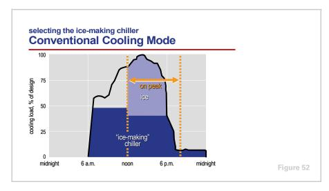
After verifying the performance of the selected chiller in ice-making mode, the next task is to consider the operation of the chiller during conventional cooling mode.
