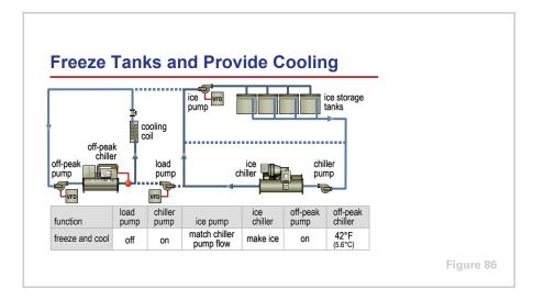
The fifth operating mode is to freeze the water inside the ice storage tanks and satisfy a simultaneous building cooling load.
