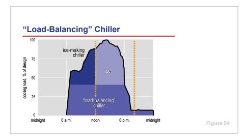
A "load-balancing" chiller is a conventional, cooling-only chiller that has just enough capacity to meet the portion of the cooling load that is not satisfied by melting ice or operating the ice-making chiller.
