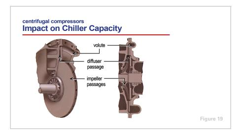
A centrifugal compressor operates on the principle of converting kinetic energy to static energy, to increase the pressure and temperature of the refrigerant vapor.
