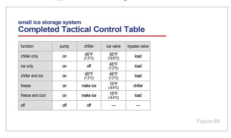
Figure 80 shows the completed tactical control table for this example small ice storage system. It describes how to accomplish each function (operating mode) by identifying the action required of each controlled component (pump, chiller, ice valve, and bypass valve) during each of the six operating modes.
