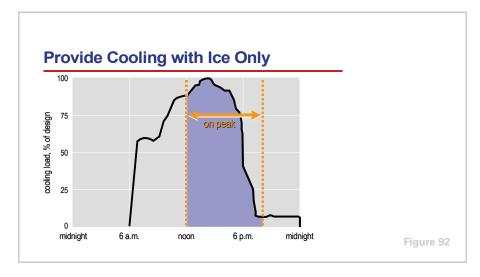
During the on-peak period, the cost of electricity is higher and there may be a demand charge. Melting the stored ice to satisfy the building cooling load,
