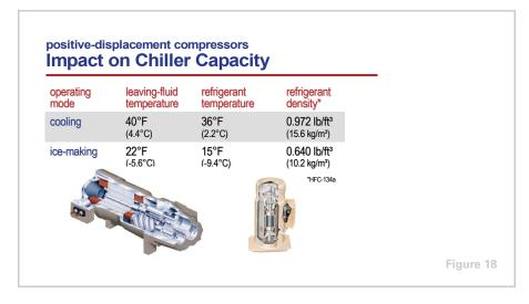
When operating in ice-making mode, an ice-making chiller has less cooling capacity than when it operates in conventional cooling mode. This loss of capacity is due to the change in density of the refrigerant vapor at the different temperatures.
