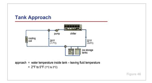
If the storage fluid inside the tank is water, the tank releases heat by changing the water from the liquid phase to the solid phase (ice). Because water freezes at 32°F (0°C), there will be no warmer temperature inside the ice storage tank during the freezing process. The temperature of the heat-transfer fluid leaving the tank will be slightly colder than 32°F (0°C). This temperature difference is called **approach**.
