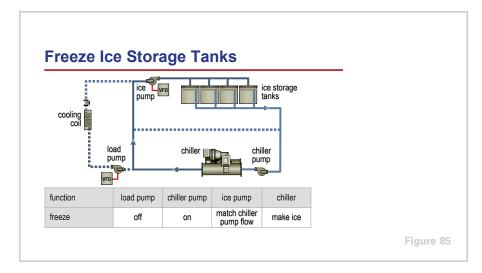
The fourth operating mode is to freeze the water inside the ice storage tanks.
