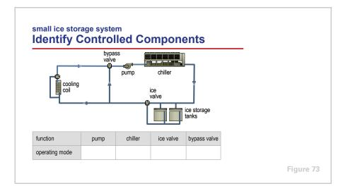
Figure 73 displays the example small ice storage system introduced in Period Four. The ice storage tanks are configured in series with, and located downstream of, the chiller.
