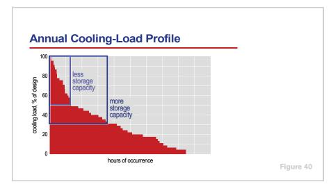
Initially, the box stretches downward faster than it stretches to the right, indicating that the on-peak demand drops faster than the installed cost increases.
