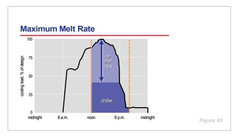
Additionally, the tanks must be selected for a melt rate that is fast enough to satisfy the portion of the design cooling load that is to be satisfied by melting the stored ice.
