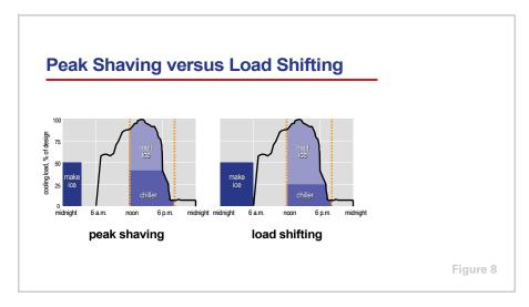
At first glance, it might appear that an ice storage system designed to reduce on-peak electrical demand (kW) is the same as a system designed to reduce on-peak electrical consumption (kWh). Which of the two is most important, however, can significantly change how the system is designed and/or controlled.
