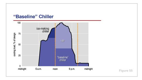
A "baseline" chiller is a conventional, cooling-only chiller that is used to satisfy a larger portion (or all) of the daily and annual cooling loads than a "load balancing" chiller. It is typically selected to be more efficient than the icemaking chiller operating in cooling mode.
