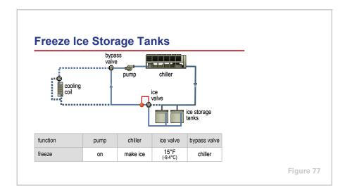
The fourth operating mode is to freeze the water inside the ice storage tanks.
