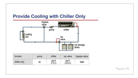
The first operating mode is to provide cooling by using the chiller alone.
