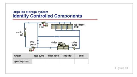
Figure 81 displays the example large ice storage system introduced in Period Four. The ice storage tanks are again configured in series with the chiller, but in this example, they are located upstream of the chiller.
