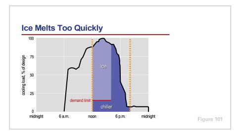
On the other hand, if the ice melts too quickly, it may be used up before the end of the on-peak period. This would cause the chiller to need to operate at a significantly higher capacity than necessary at the end of this period.
