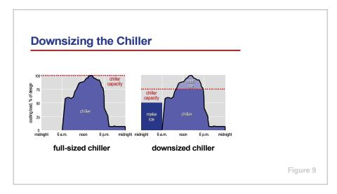
In addition to lowering monthly utility costs, another potential benefit of ice storage is to reduce the size and capacity of mechanical cooling equipment.
