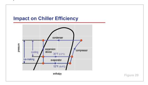
Additionally, when operating in ice-making mode, an ice-making chiller will generally be less efficient than when it operates in cooling mode.
