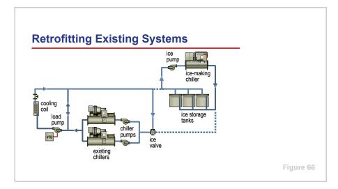
During the off-peak period, the ice valve diverts all the fluid returning from the cooling coils to bypass the tanks, isolating the tanks and ice-making chiller in a separate loop. The ice pump circulates the heat-transfer fluid through the ice-making chiller and storage tanks, freezing the water inside the tanks.
