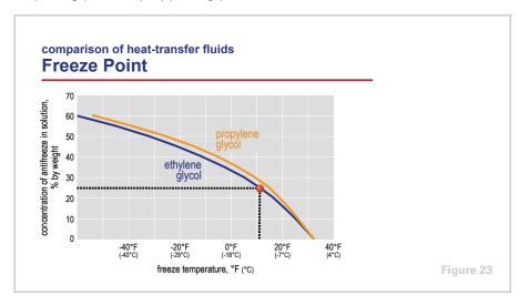
Propylene glycol offers slightly less freeze protection than ethylene glycol. Therefore, a higher concentration of propylene glycol is required to achieve the same freeze point.
