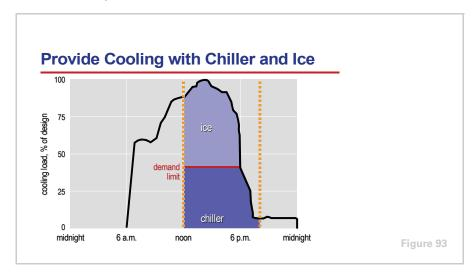
In a partial-storage system, the portion of the on-peak cooling loads satisfied by the chiller is regulated by limiting the capacity of the chiller, often referred to as demand limiting. The cooling loads above this demand-limited capacity of the chiller are satisfied by melting the stored ice. In the example shown in Figure 93, the chiller satisfies about 40 percent of the design cooling load during the on-peak period, and the ice is melted to satisfy the remainder of the loads.
