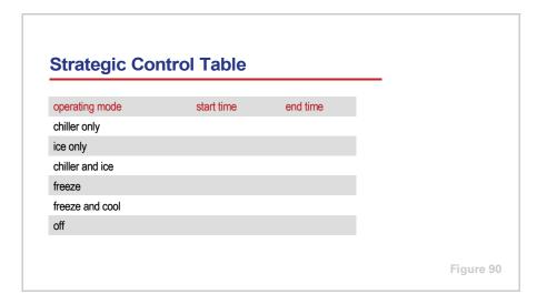
After the on-peak and off-peak periods have been determined, the next step is to identify the time of day that each of the system operating modes will begin and end.
