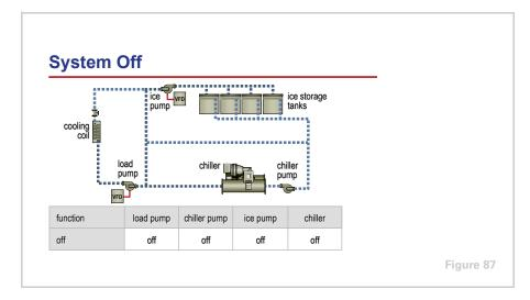
The final operating mode, turning the system off, is used when no building cooling load exists, and all the water inside the ice storage tanks is frozen. All three pumps and the chiller are off.
