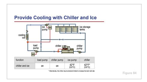
The third operating mode is to provide cooling by operating the chiller and melting ice simultaneously.
