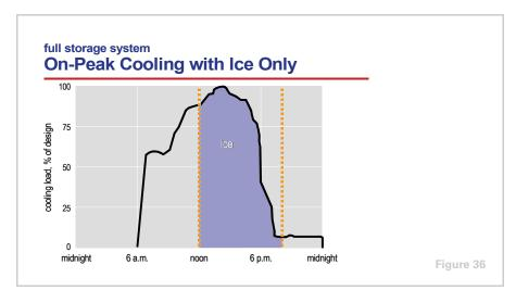
As discussed in Period One, one approach is to design a full-storage system with sufficient ice storage capacity to satisfy the entire on-peak cooling
