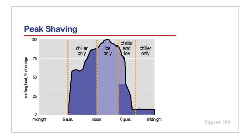
On the example day shown in Figure 104, there is sufficient ice storage capacity to meet most of the on-peak cooling loads, but not enough to meet the loads throughout the entire on-peak period. Therefore, the system uses the "ice only" operating mode between noon and 4 p.m.
