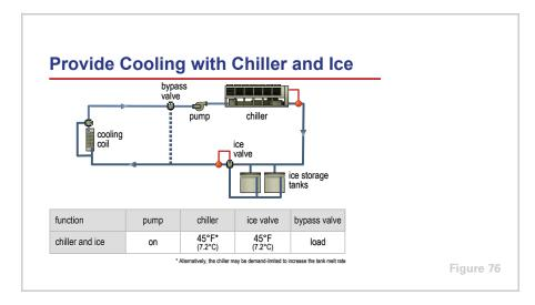
The third operating mode is to provide cooling by operating the chiller and melting the ice simultaneously.
