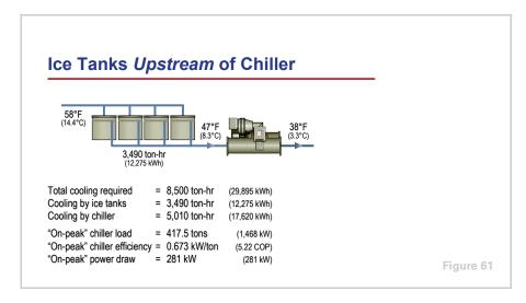
Now, consider if the ice storage tanks are located *upstream* of the chiller, instead of downstream. This configuration allows the tanks to receive the warmest entering-fluid temperature and operate at a higher leaving-fluid temperature. This results in increased storage capacity.
