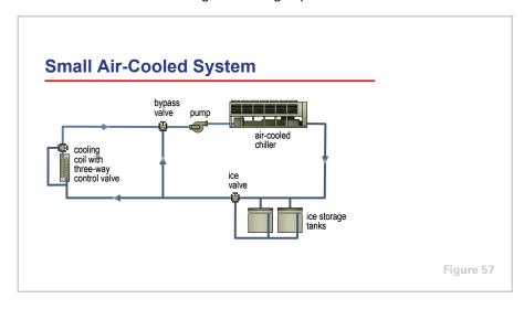
Most ice storage systems are used in smaller buildings. In these smaller systems, the equipment layout is similar to that shown in Figure 57. This popular system configuration requires a single constant-volume pump to circulate the heat-transfer fluid through the chiller, ice storage tanks, and cooling coils. Because this is a constant-flow system, the capacity of the cooling coil is modulated with a three-way control valve. (For clarity, only a single cooling coil is shown.)
