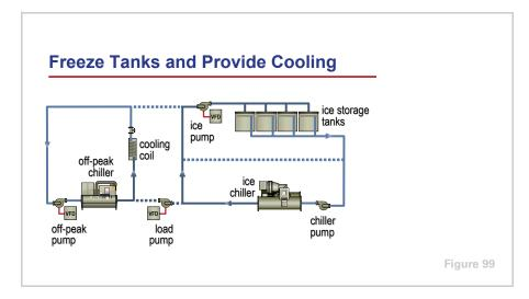
If the building cooling loads that exist during the time when the system is to be making ice are significant, it is typically advantageous to use a separate, "offpeak" chiller to satisfy these loads. The ice-making chiller is less efficient when making ice. This configuration allows the ice-making chiller to be used only for the purpose of making ice, allowing it to use its full capacity to freeze the water inside the tanks as quickly as possible.
