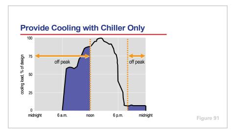
During the off-peak periods, the cost of electricity is lower and there is often no demand charge. With low-cost electricity, operating the electrically powered chiller is typically the most economical means of satisfying the building cooling load.
