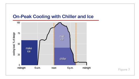
The installed cost of a full-storage system, however, may not be feasible. Many ice storage systems have enough capacity to satisfy only a portion of the onpeak cooling loads. This type of system is often called a "partial-storage system."
