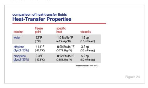
Because propylene glycol has a slightly higher specific heat than ethylene glycol, it would appear that the fluid flow rate required with propylene glycol would be slightly less. Unfortunately, this does not equate to reduced pumping power or better heat transfer, because propylene glycol has a substantially higher viscosity than ethylene glycol. This means that a system using propylene glycol will require larger pumps, and potentially larger cooling coils, due to the loss of heat transfer.
