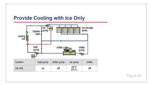
The second operating mode is to provide cooling by melting the ice alone.
