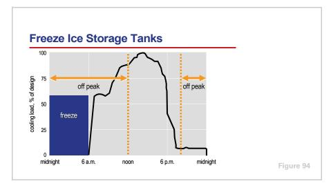
As mentioned previously, ice storage systems shift operation of the electrically powered chiller to off-peak periods, when it can freeze the water inside the ice storage tanks while the cost of electricity is low.
