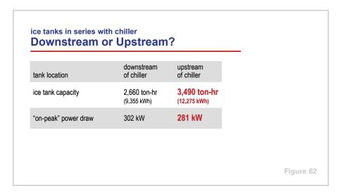
Locating the 20 ice storage tanks upstream of the chiller, rather than downstream, reduced the on-peak electrical demand by an additional 21 kW.
