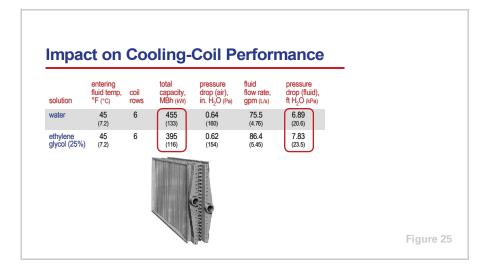
The negative impact on heat transfer that results from adding antifreeze to the heat-transfer fluid can be illustrated by examining the performance of a cooling coil. Figure 25 shows the performance of an example cooling coil that contains six rows of tubes with 118 fins/ft. This coil has been selected for an airflow of 12,000 cfm (5,663 L/s) and a total cooling capacity of 455 MBh (133 kW).
