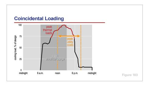
If the primary mission of a partial-storage system is to reduce on-peak electrical demand (kW), ice storage typically provides its greatest economic benefit when the building cooling load, the cost of electricity, and the building electrical load all peak simultaneously.
