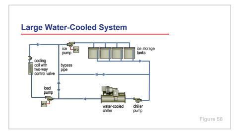
As an ice storage system gets larger, the opportunity to optimize pump power is often justified. This is accomplished by using three separate pumps, each with its own specialized duty. In the example, larger system shown in Figure 58, the constant-volume **chiller pump** is sized to deliver the design system flow rate, but with only as much head as required to overcome the pressure drop of the chiller evaporator.
