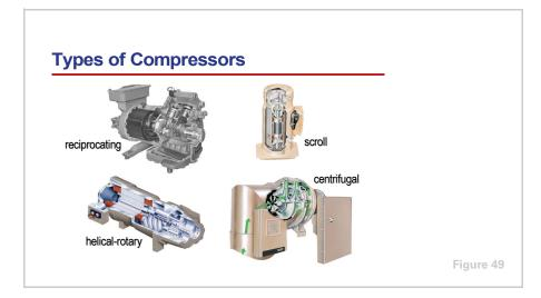
Chillers that include helical-rotary, scroll, or reciprocating compressors are typically suitable for ice-making duty without modification. Again, these positive-displacement compressors will operate at reduced capacity and reduced efficiency when producing colder fluid temperatures during ice-making mode.
