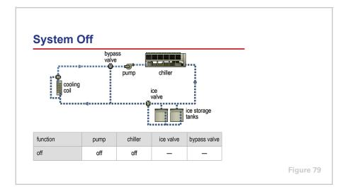
The final operating mode, turning the system off, is used when no building cooling load exists, and all the water inside the ice storage tanks is frozen.
