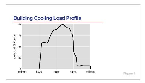
Adding ice storage to an HVAC system can reduce the utility costs associated with cooling by shifting the operation of the chiller from times of high-cost electricity to times of low-cost electricity.
