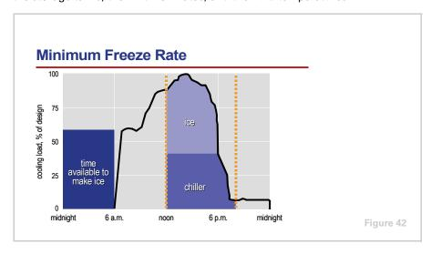
The ice storage tanks must be selected for a freeze rate that is fast enough to make the desired amount of ice in the time available for ice making. This minimum freeze rate also dictates the required capacity of the chiller when it operates in ice-making mode.
