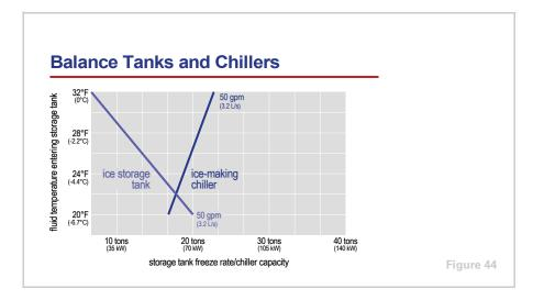
Decisions made when selecting the chillers, the ice storage tanks, and the system flow rates and temperatures are interrelated. As described in Period Two, the ice storage tank and the chiller respond differently to various fluid flow rates and temperatures. For example, as depicted in Figure 44, colder fluid temperatures increase the freeze rate of an ice storage tank, but decrease the ice-making capacity of the chiller.
