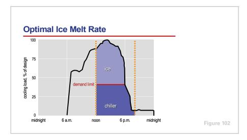
In this last example, the chiller is demand-limited to operate at a capacity that allows the ice to melt at the optimal rate, ensuring that all the ice is melted by the end of the on-peak period.
