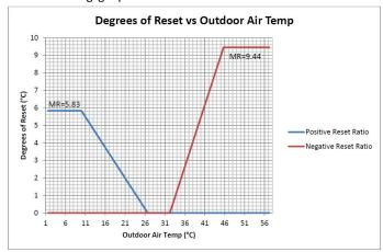
The following graph shows the reset function for Return Chilled Water Reset:
