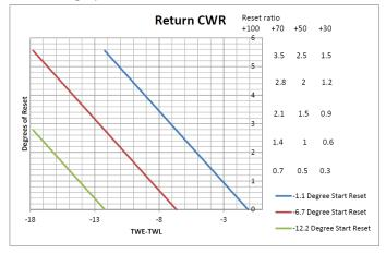
TWE-TWL is the difference between the evaporator entering water temp and the evaporator leaving water temperature.
