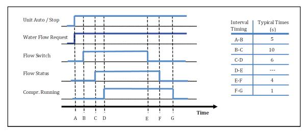
If water flow is not established in 20 minutes (for normal transition), the UC800 de-energizes the Pump relay and generates a non-latching diagnostic. If flow returns (e.g. someone else is controlling the pump), the diagnostic is cleared, the Pump is re-energized, and normal control resumed.
