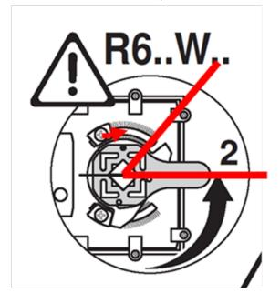
If the minimum opening is modified after the first powering, motor re-calibration is needed to validate the new operating range. When motor is powered, push green led button (2). Motor memorizes the new reference of end of travel position on its signal (2...10 VDC)
