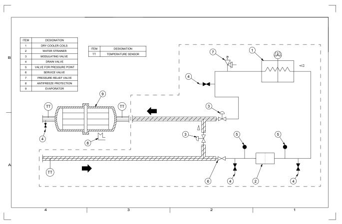
Note: glycol free cooling chilled water setpoint should be in the range of [4°C - 20° C]. Water & Glycol mixture is filled on the free cooling coils on valve item 4 (3/4'').
