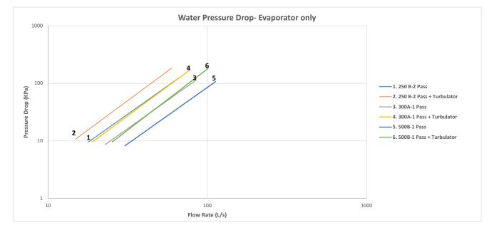
Figure 16 – Evaporator water pressure drop
