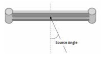
To avoid damage from the spray wand contacting the coil, make sure the  $90^{\circ}$  attachment does not come in contact with the tube and fin as abrasion to the coil could result.
