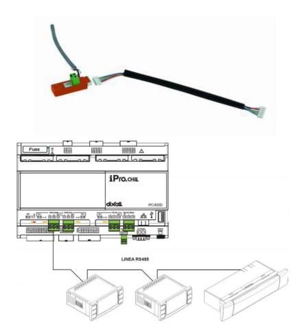
To connect to the devices to be controlled simply use two minimum cross-section of 0.5 mm<sup>2</sup> plus screen, use the input GND only for communication problems.
