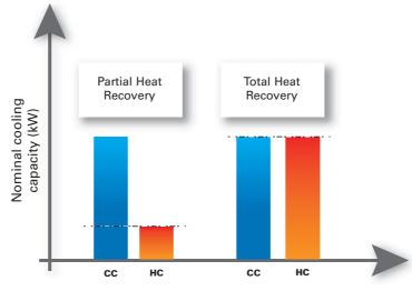
CC = Cooling capacity HC = Heating capacity
