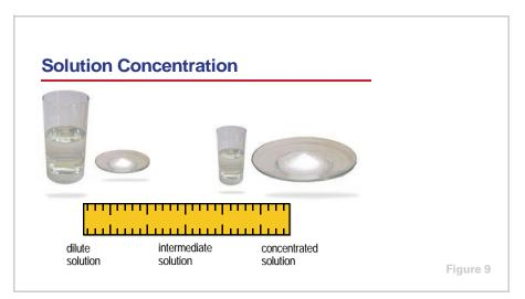
These two fluids, the refrigerant and the absorbent, are mixed inside the chiller in various concentrations. The term **dilute solution** refers to a mixture that has a relatively high refrigerant content and low absorbent content. A **concentrated solution** has a relatively low refrigerant content and high absorbent content. An **intermediate solution** is a mixture of dilute and concentrated solutions.
