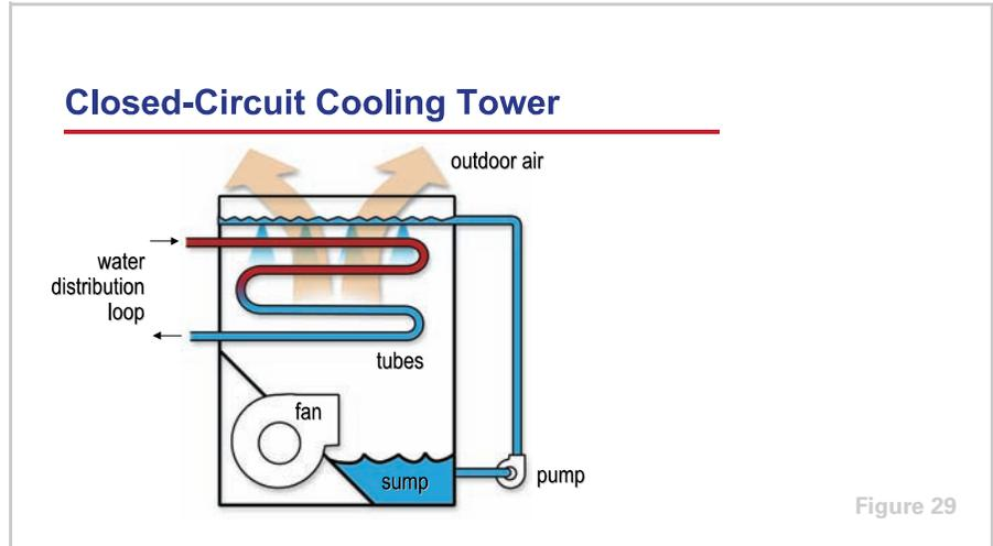
In a **closed-circuit cooling tower**, warm water from the water-source heat pump distribution loop travels through closed tubes inside the cooling tower, while air is drawn or blown over these tubes by a fan. Water is pumped from the tower sump and sprayed over the tube surfaces. As the air passes over the tubes, it causes a small portion of the water on the outer tube surfaces to evaporate. This evaporation process absorbs heat, cooling the water inside the tubes.
