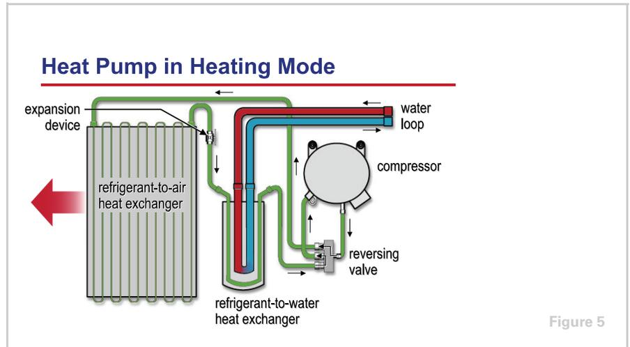
A heat pump includes a reversing valve that allows it to also function in the heating mode.
