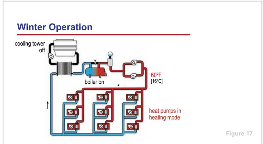
During cold weather, when most of the heat pumps are operating in heating mode, heat is removed from the water loop and transferred to the air. This causes the temperature of the water in the loop to drop, making it necessary to add heat to the water loop. A boiler or water heater adds heat to the water loop, maintaining a leaving-water temperature of approximately 60°F [16°C].
