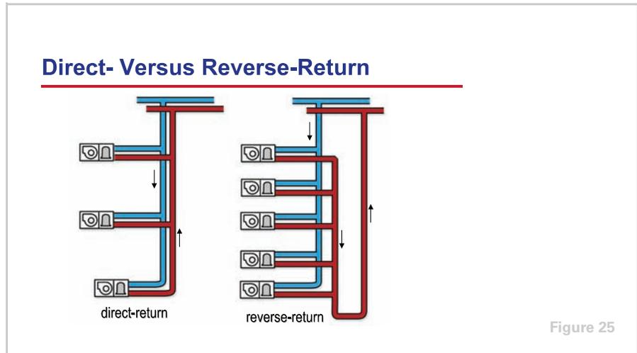
The water distribution loop should be designed to deliver the required water flow to each heat pump while minimizing pump energy and noise problems. Because distribution-loop piping can account for 25 percent to 35 percent of the total system installation cost, careful planning of the piping arrangement is important.
