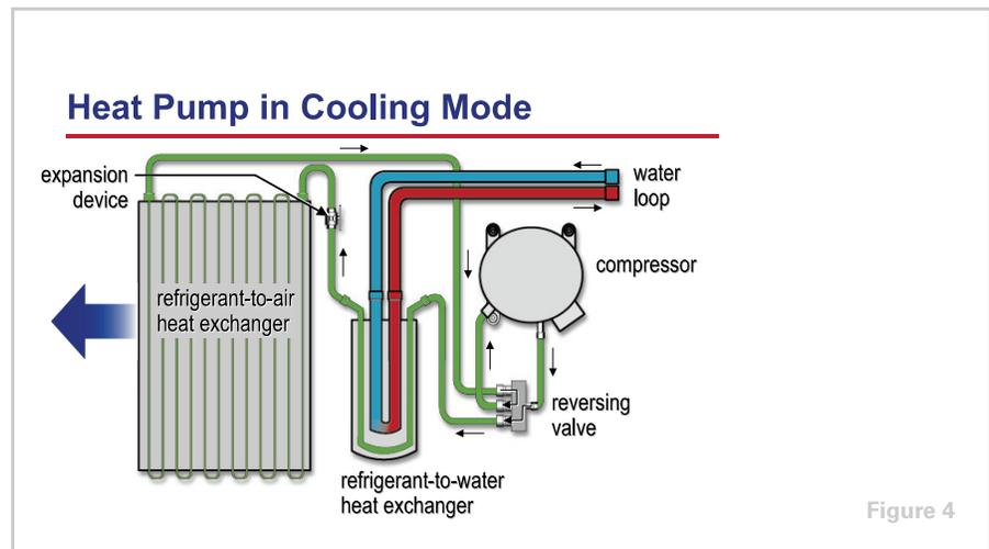
A heat pump is basically a device that transfers heat from one substance to another substance. It has these same basic refrigeration components: compressor, condenser, evaporator, and expansion device. The difference is that it can also reverse the refrigeration cycle to perform heating, as well as cooling, by reversing the functions of the two heat exchangers. The operation of the refrigeration cycle changes depending on whether the unit is in cooling or heating mode.
