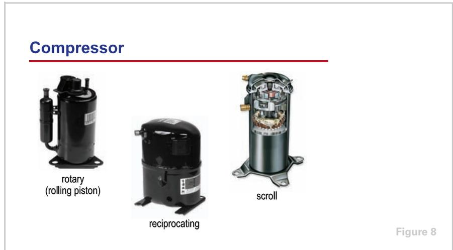
Each heat pump includes at least one **compressor**. Some higher-capacity models may use multiple compressors. Depending on its size and manufacturer, this compressor may be rotary (rolling piston), reciprocating, or scroll type. The selection of the type of compressor generally depends on the capacity and electrical requirements of the heat pump.
