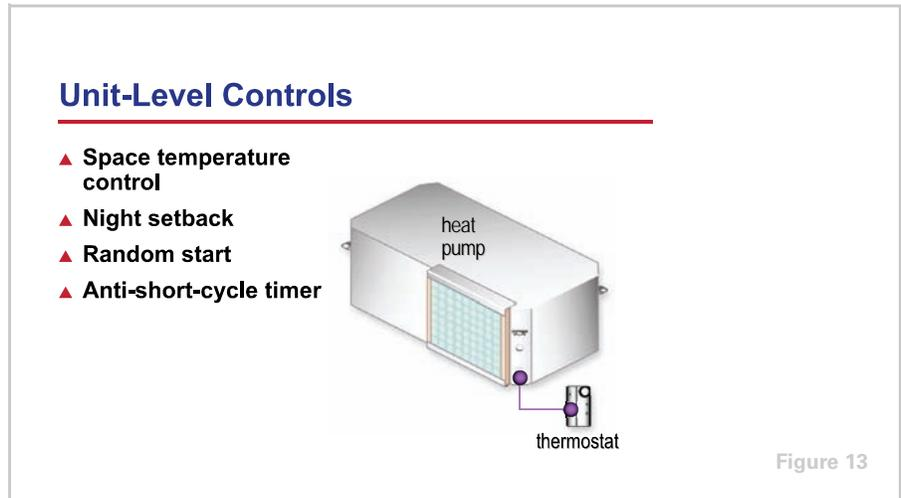
Each space or zone in a building is served by a heat pump. Each heat pump must be able to respond to the cooling or heating demands of its space. This is often accomplished by using a conventional thermostat to control the operation of the heat pump.
