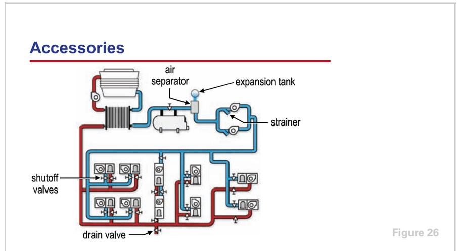
There are typically several other accessories included in the water distribution loop. These include strainers, an air separator, an expansion tank, drain valves, shut-off valves, balancing valves, and flow indicators.
