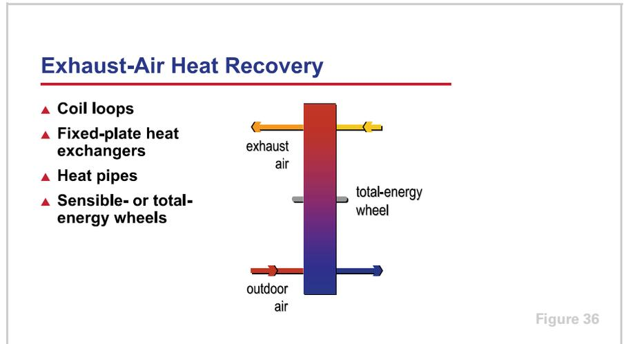
A centralized ventilation system makes it possible to implement exhaust-air heat recovery to precondition the outdoor air. In applications where the exhaust air from the building can be routed back to a central location, exhaust-air heat recovery is a very effective means of reducing the ventilation load and saving energy.
