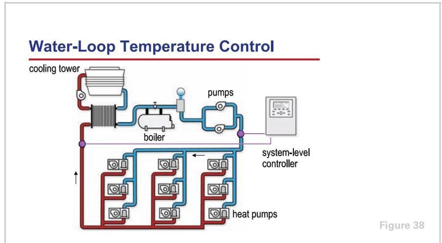
As mentioned earlier, water-source heat pumps can run in either heating or cooling mode when the water loop temperature is maintained between 60°F [16°C] and 90°F [32°C]. Loop temperatures that are outside the recommended range can severely impact heat pump performance. For this reason, the primary function of a system-level controller is to monitor and maintain an acceptable temperature in the water loop.
