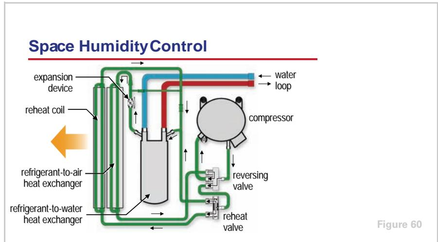
One cost-effective method of controlling space humidity is to temper the cool supply air with heat that is recovered from the heat-pump refrigeration circuit. This is sometimes referred to as hot-gas reheat. In this configuration, the air is first cooled by the refrigerant-to-air heat exchanger, then tempered by the reheat coil to control not only the dry-bulb temperature, but also the relative humidity of the space.
