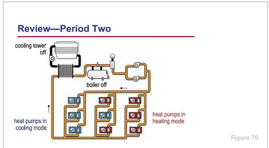
Period Two reviewed the operation of a traditional cooling-tower-and-boiler, water-source heat pump system during the different seasons of the year. This discussion revealed the heat-recovery nature of this system, as it uses heat removed from internal spaces to provide heat to perimeter spaces. This heat recovery offers the potential for energy savings during much of the year. Other benefits of the water-source heat pump system include:
