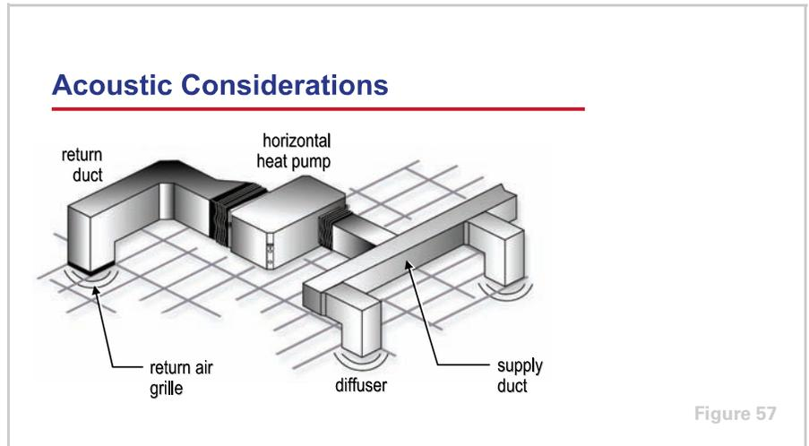
For heat pump configurations that use ductwork to deliver air to the space, such as horizontal, vertical, rooftop, and some vertical-stack heat pumps, the design of the supply-and-return air distribution systems is critical for ensuring proper space acoustics. The example system shown in Figure 57 includes the following features that help reduce the amount of noise that reaches the occupied space.
