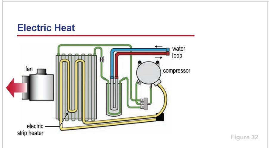
An alternative to including a heat adder, such as a boiler, in the system is to install an electric strip heater either inside the heat pump or in the downstream ductwork. In this configuration, the heat pump operates in normal heating mode until the temperature of the water in the loop falls below approximately 60°F [16°C]. At that point, the compressor turns off and the electric strip heater is energized to warm the air.
