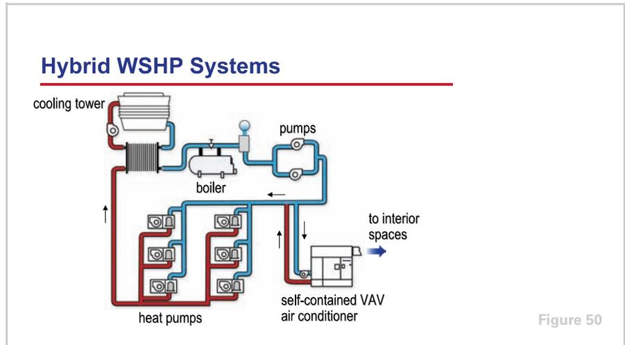
This second example hybrid system, shown in Figure 50, uses variable-air-volume (VAV), self-contained air conditioners to serve the interior spaces of the building and water-source heat pumps to serve the perimeter spaces. The interior spaces in this example have variable loads, but always require cooling.
