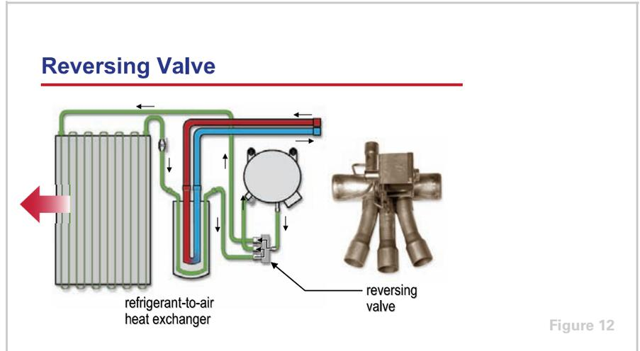
The **reversing valve**, sometimes called a four-way valve, is the component that allows the heat pump to perform heating as well as cooling. It is called a reversing valve because it is used to reverse the direction of refrigerant flow through the cycle. In the heating mode, refrigerant vapor from the compressor is diverted by the reversing valve to the refrigerant-to-air heat exchanger. In this heat exchanger, heat is transferred from the refrigerant vapor to the air, heating the air.
