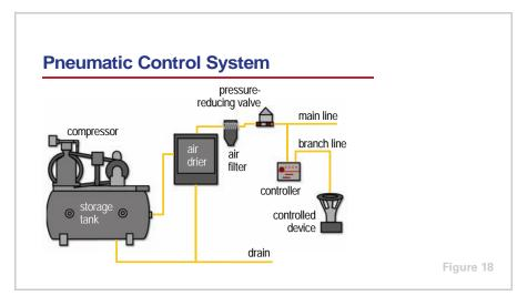
**Pneumatic** control systems vary the pressure of compressed air to operate controlled devices, such as valve and damper actuators. Pneumatic control systems consist of the following major components:
