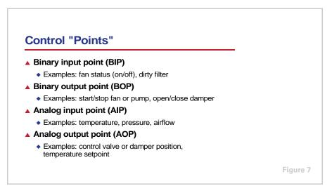
A control point is an individual input to, or output from, a controller. The term binary refers to a control signal that has only two possible states, such as on or off. Examples of binary input points (BIP) include a switch that indicates whether a fan is on or off, and a pressure limit switch that indicates when a filter
