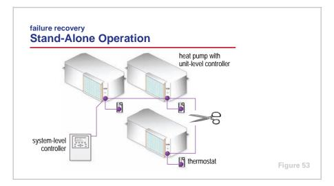
As mentioned earlier, one of the benefits of a distributed control architecture is that it allows stand-alone control of each piece of equipment. In the event that communication with the system-level controller is lost, the unit-level controller should contain a set of instructions and setpoints that would protect the piece of equipment and allow it to continue providing cooling or heating.
