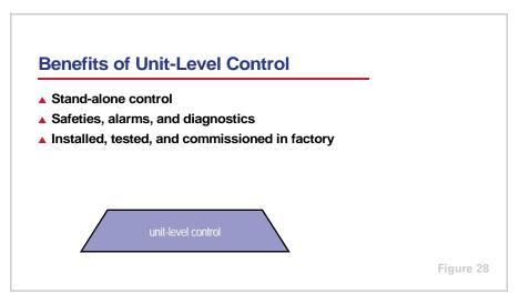
The primary focus of this clinic will be on using a separate piece of hardware to provide unit-level and system-level control functions. This type of distributed architecture provides several benefits. The first is that it allows stand-alone control of each piece of HVAC equipment. This improves the reliability of the system, because the unit-level controller can control and protect the equipment even if communication from the system-level controller fails.
