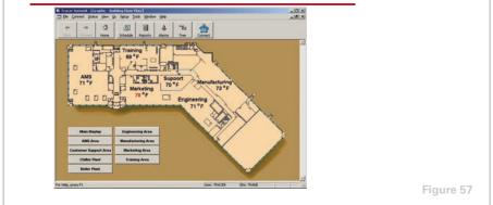
Linking all of the system-level controllers to a building automation system, however, allows the building operator to quickly and efficiently respond to comfort-related complaints from a central location.
