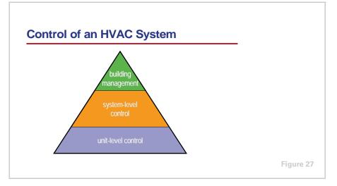
For the purposes of this clinic, automatic control of an HVAC system will be separated into the three levels depicted by the pyramid in Figure 27. The base of the pyramid is formed by the unit-level control of each individual piece of HVAC
