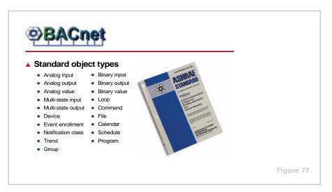
Interoperability at the unit-control and building-control levels is important to the overall flexibility of the BAS infrastructure, as well as for competitive procurement. Today, within the building automation industry, there are two dominant open, standard protocols used to provide interoperability at these two levels.
