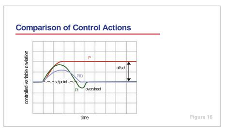
As a review, this illustration shows the variation of the controlled variable from the setpoint. With proportional (P) control, the corrective action is proportional to the magnitude of the deviation from the setpoint. The condition of the
