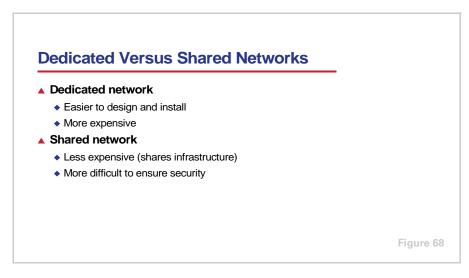
Historically, most building automation systems have been installed on **dedicated networks**. This means that the communications media is used only by the building automation system, and not shared with other systems such as telecommunications or e-mail. Dedicated networks are easier to design and install because they do not need to consider the needs or limitations of these
