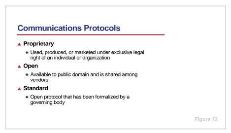
In order for microprocessor-based devices to communicate with one another, they need to "speak a common language." A **communications protocol** is a set of rules or standards that govern the exchange of data over a digital
