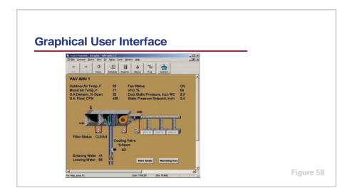
Graphical representations of the HVAC equipment and systems often make it easier to navigate the system when investigating problems. This is because the graphics on the screen mimic what the operator knows to be installed on the roof, in the equipment rooms, and in the ceilings.
