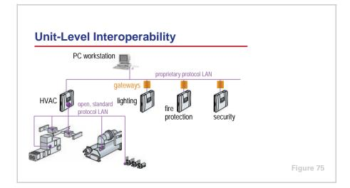
In this second scenario, unit-level controllers provided by manufacturer A are used to control the VAV terminal units. The unit-level controllers on the other pieces of HVAC equipment, and the system-level controller, are provided by manufacturer B. By using an open, standard communications protocol at the unit control level, the unit-level controllers on the VAV terminal units can communicate with the HVAC system-level controller without the need to install a gateway.
