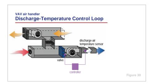
Unit-level control for a piece of HVAC equipment typically involves the use of several control loops. To demonstrate this, assume that the same example cooling coil that was introduced in Period One is installed inside a variable-air-volume (VAV) air handler. This air handler delivers a variable quantity of constant-temperature air down the supply-duct system.
