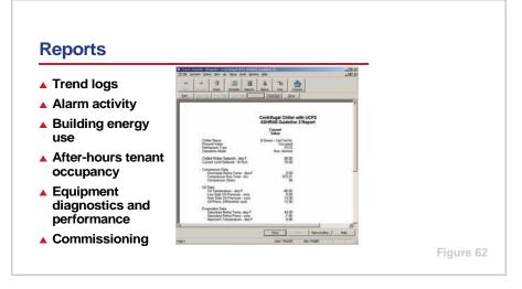
Many of the benefits of a building automation system come from taking advantage of the processing power and data storage capacity of the PC. Microprocessor-based control systems have the capability of gathering and transmitting large quantities of data. Presenting this data in an easy-to-use format is critical to ensuring that it is useful to the operator.
