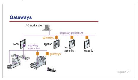
In the past, due to the lack of open, standard communications protocols, manufacturers of microprocessor-based building automation systems developed their own unique, proprietary protocols for communicating information between unit-level and system-level controllers, and between system-level controllers and the building automation system. These proprietary protocols resulted in customers being limited to buying from a single manufacturer when they wanted to expand the system.
