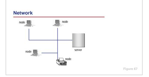
A **network** is the means by which two or more communicating devices are connected together so they can exchange data. Physically, the connections can be made with cables or through a wireless network.
