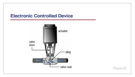
Similar to the pneumatically-controlled valve, the body of a valve used in an analog-electric control system also contains a plug that travels up and down to vary the flow of water through the valve. The difference is in the valve actuator.
