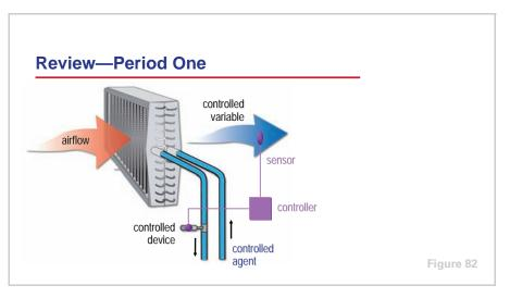
Period One introduced the concept of the control loop, using a chilled-water cooling coil as an example. A control loop consists of a controlled variable, a sensor, a controller, a controlled device, and a controlled agent.
