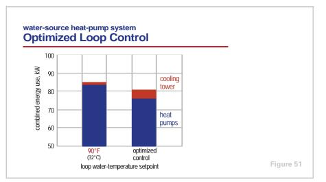
In the example water-source heat pump system, a communicating system-level controller offers the opportunity to optimize the temperature of the water in the loop, minimizing total system energy consumption.
