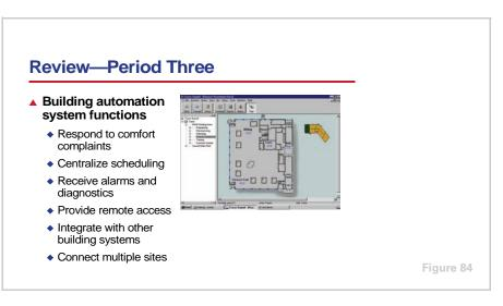
The combination of unit-level and system-level control can provide a functional operating HVAC system for a building. However, operators frequently want to monitor the building, receive alarms and diagnostics at a central location, centralize scheduling functions, and integrate the HVAC system with other building systems. These are some of the functions, which are provided by a building automation system, that were discussed in Period Three.
