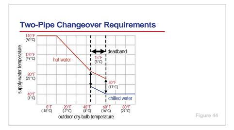
Changing between cooling and heating modes in a two-pipe system requires a lot of excess energy to heat or cool the mass of water in the piping system. Therefore, ASHRAE Standard 90.1–2001 (Section 6.3.2.2.2) includes the following requirements to minimize the energy impact of this switchover:
