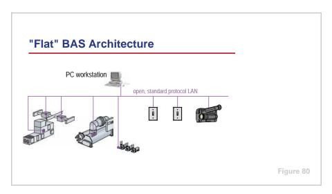
An alternative to tiered architecture uses an open, standard protocol to flatten out the BAS architecture, by connecting the unit-level controllers directly to the main LAN. This approach may reduce hardware costs by eliminating the system-level controllers, but requires the system-coordination logic (scheduling, trending, and optimization routines) to be scattered throughout the network.
