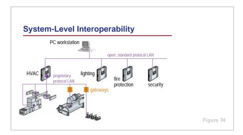
As stated at the beginning of this period, **interoperability** is defined as digital communication between independently manufactured products that are designed to the same open, standard communications protocol. It means that a single controller can monitor and control independently designed microprocessor-based control products.
