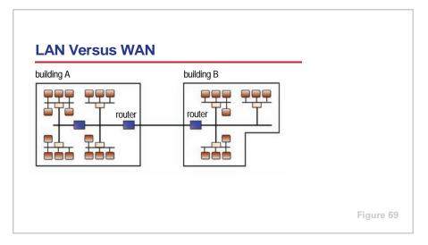
A **local area network (LAN)** is a communications network that is intended to serve a relatively small area, typically up to approximately one square mile (2.5 square kilometers). Because the network serves only a small area, it can be optimized to allow faster exchange of data. A LAN generally works well for a single building.
