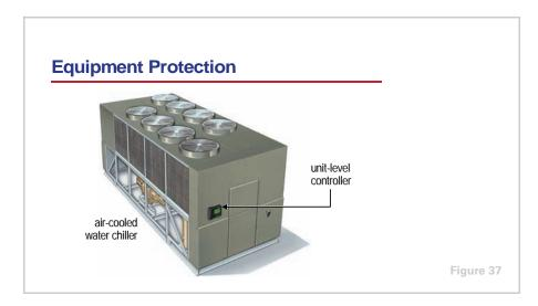
As described earlier, another important function of a unit-level controller is to protect the equipment from damage. As an example, Figure 37 shows an aircooled water chiller with a microprocessor-based unit controller. Suppose a condenser fan motor fails during hot weather. With less air flowing through the air-cooled condenser, the temperature (and pressure) of the refrigerant inside the condenser gradually rises.
