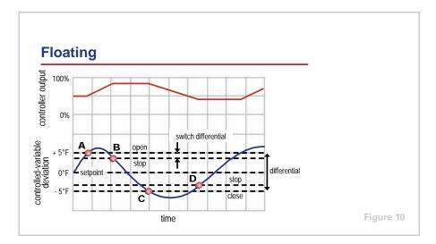
A variation of two-position control is **floating** control, sometimes called threeposition control (open-stop-close). Typically, floating control uses a slowmoving actuator and a fast-responding sensor. The controlled device either modulates toward the open position, modulates toward the closed position, or holds its current position.
