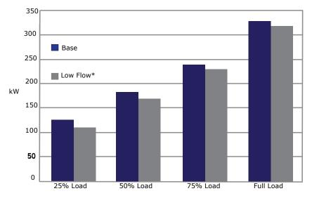
Figure 21. Chilled water system performance at part load
