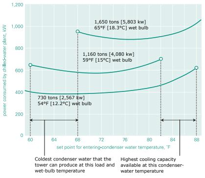
Figure 54. Chiller-tower energy consumption
