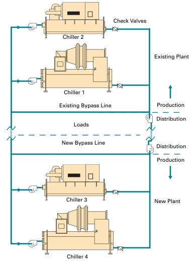
Figure 36. Double-ended decoupled system
