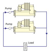
Figure 10. Manifolded pumps
