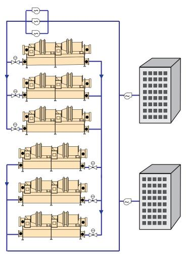
Figure 19. Large chilled-water system schematic
