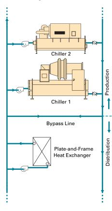
Figure 40. Sidestream plate-and-frame heat exchanger
